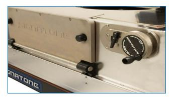
Platen "Fine Adjust" and "Position Lock"
